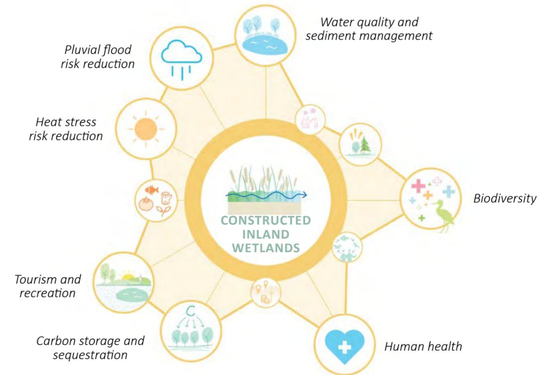
**Pluvial flood risk reduction:** Constructed inland wetlands collect urban stormwater runoff during storm events. While their flood attenuation benefits may vary, they typically include a flood bypass channel to prevent damage to the wetland during major flood events. As such, their flood mitigation potential is typically most optimal for small flood events.
