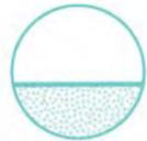
**Soil:** Soil for bioretention areas typically include mixed soils or engineered media. High infiltration rates of the media are key. To ensure drainage capacities, well-draining soils are often considered during the design. The underlying soils typically have low infiltration rates and as such, underdrains can be part of the design (DDOE 2012; MSW 2018).
