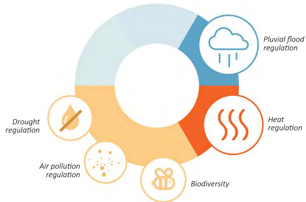
**Pluvial flood regulation:** Green roofs capture and store rainwater in the soil and in the roof construction and thus, reduce peak stormwater load on stormwater and sewerage systems. Standards capacities range depending on the type of green roof (see section Special Techniques), varying from 20–50 l/m<sup>2</sup> for extensive green roofs to 30–160 l/m<sup>2</sup> for intensive green roofs (Eisenberg and Polcher 2020).
