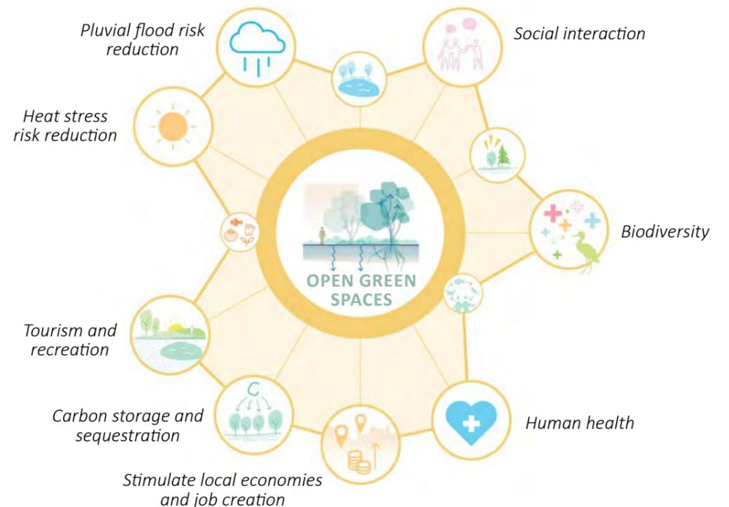
**Pluvial flood risk reduction:** Open green spaces reduce the impact of storms and can decrease potential damage to buildings and infrastructure. To achieve a greater cumulative effect, a series of green open spaces should be planned as a coherent blue-green infrastructure network that can absorb, infiltrate, and store large volumes of stormwater and reduce the velocity of stormwater flow in large parts of the city. (Gehrels et al. 2016).
